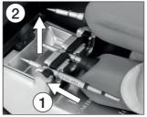
Push the cartridge into the tool to the mark\*.
