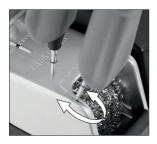
Fit the tip into the aligner and turn to the desired position.
