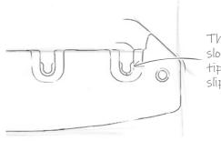
The extractor slot prevents tips from slipping
