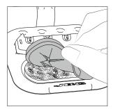
Lift the wiper membrane by using the recess on the edge. Remove the wiper and replace the brass wool with a new one. Make sure that the brass wool is on the far left and that there is space for the wiper on the right.
