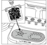
CL0300 Brass Wool is a very effective cleaning method. It leaves a small layer of solder on the tip, preventing oxidation between cleaning and rewetting.
