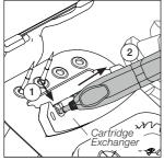
Place the tool with the cartridge over the cartridge exchanger slots and press down (1) until it clicks. To remove the cartridge pull the handle out (2).
