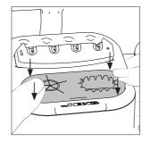
Press the wiper membrane down at the 4 corners until you feel it click into place. Make sure that the wiper
