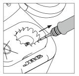
Use the slots to remove remaining particles.
