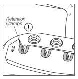
The cartridge exchanger allows inserting / changing cartridges safely without switching the tool off. Cartridges are held in place thanks to the retention clamps (1).
