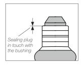
Make sure the sealing plug is placed correctly.
