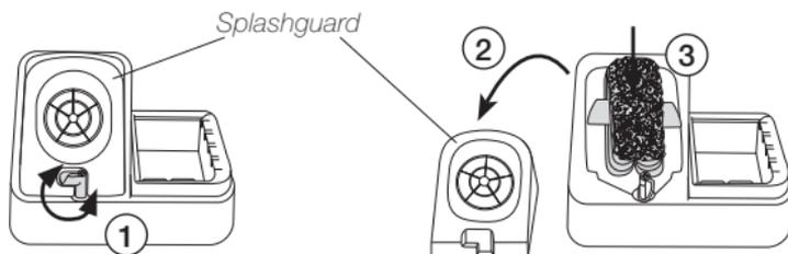
Open (1) and remove (2) the splashguard. Insert the metal brush set (3). The clip must come to rest at the rear end. Finally reassemble the splashguard.
