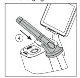
Place the tool in the charging holder (4) to charge it. A beep will sound when the tool is properly placed and charging. The volume can be adjusted using the left button on the display.
