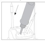
Place the handle on top of the new cartridge and press down.
