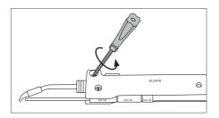
Unlock the cartridge fixing screw.
