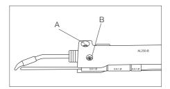
Lock the Cartridge fixing screw (A) and the guide tube screw (B).
