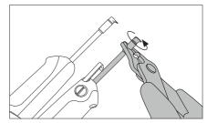
Align cartridges with JBC pliers.
