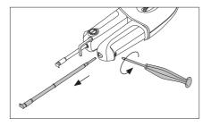
Loosen the screws and remove the cartridges.
