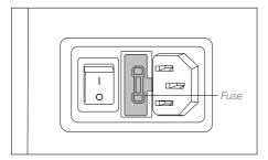
2. Press the new fuse into the fuse holder and replace it in the station.
