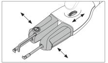
The wheel allows to adjuste the wire stripper arm position accordig to the wire diameter. Move the wheel backward for a wider and forward for a narrower position.
