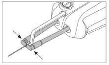
Choose cartridges according to the wire diameter. Pinch the wire with the blades. The pinched area will be melted by heat.
