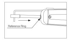
Insert the cartridge until the reference ring touch against the wire stripper. Take the ring as reference and check that both tips match.
